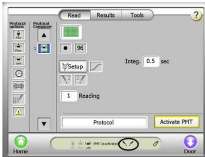
13. Power on the instrument which automatically powers the Injector System. Go to the INSTRUMENT CONTROL screen, touch the **READ** button. Installation is successful if an **INJECTOR** icon appears on the **INSTRUMENT STATUS** bar. If no **INJECTOR** icon appears, verify that the DB-15 cable is securely connected to the correct port on the back of the instrument. Contact technical support if further assistance is needed.
