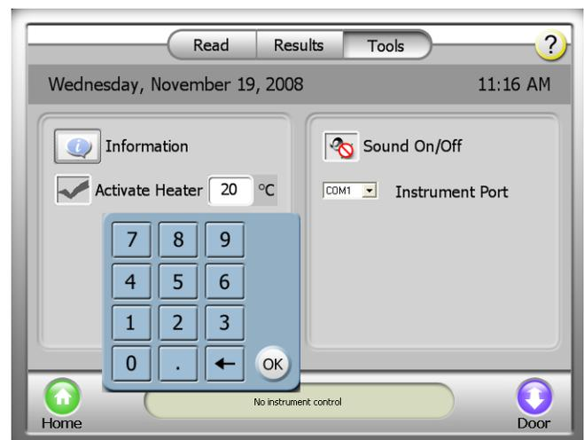
**Figure 7-1: Accessing the Heater Option via the TOOLS Button**
