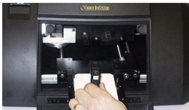
Figure 3-1: Installing a Fluorescence Optical Kit
