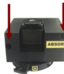
Figure 4-8: Arrows Point to the Two Captive Screws on the Absorbance Module
