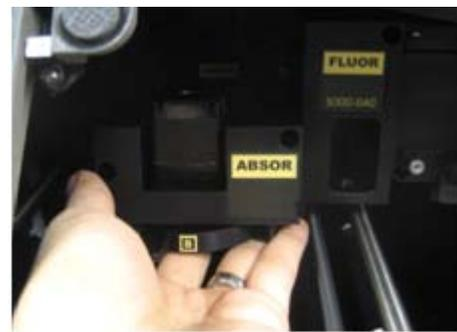
Figure 4-7: Installing the Absorbance Module
